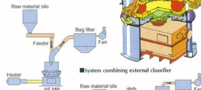
■Drying and grinding system
